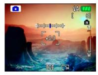
2. Use the **Left/Right** to adjust the exposure value for the picture. The range is from EV -2.0 to EV+2.0 (steps of 0.3).
